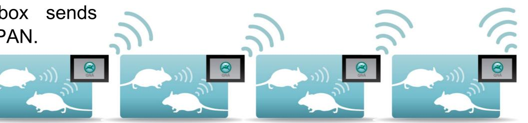
The RF transmission is done through a custom-made protocol that uses a 500kHz output frequency to send the ID, temperature bandwidth and losses due to the data and CRC. In transmission mode the average current consumption is 2.5mA. The receiving antenna placed under the cage in the experiments measured 250x350mm.
